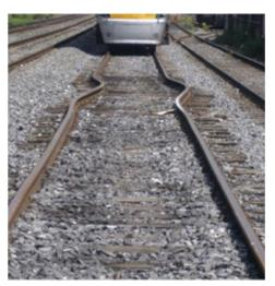
inevitable consequence is a derailment. Speed restrictions may have to be imposed where the network operator believes there is a risk of buckling. This has a knock-on effect on the timetable and will result in loss of revenue and inconvenience to the rail customers.
