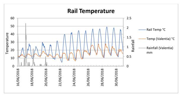
The Rail Temperature chart is compiled from Rail Temperature data collected via RailTel from an Irish Rail installation 75km to Met Eireann Valentia Observatory<sup>ii</sup>. There are a number of trends that can be seen from the chart:
