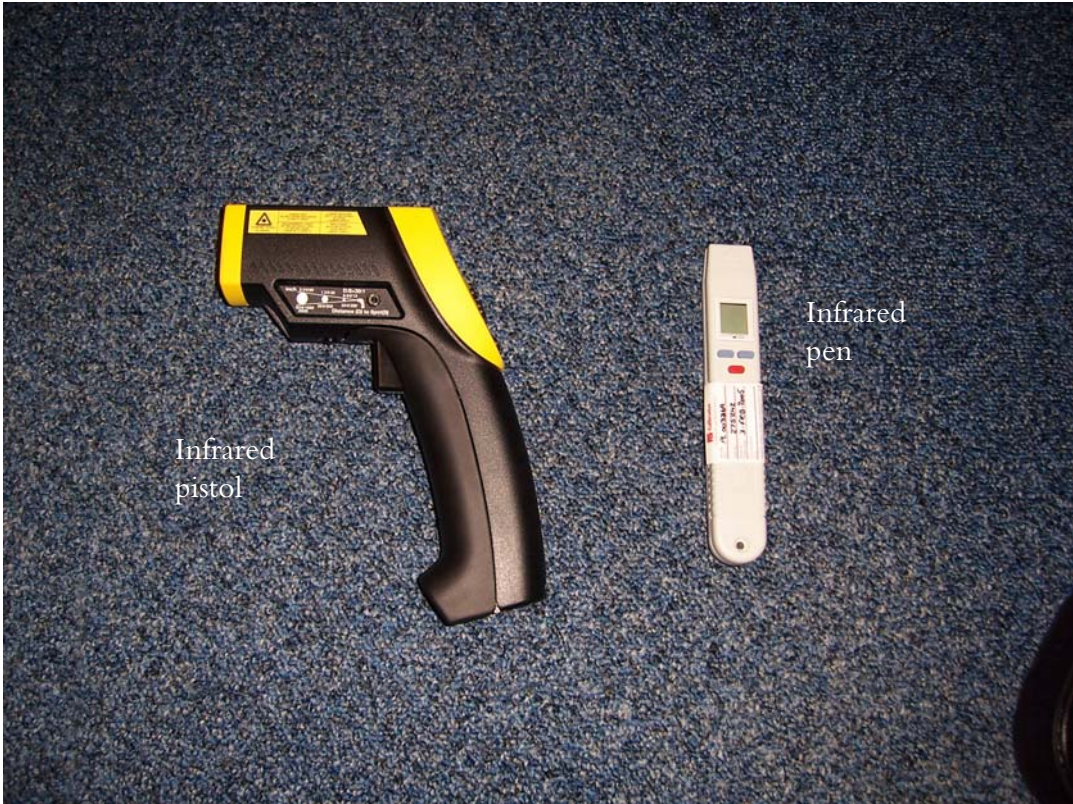
Figure 7 Two non-contact thermometers used on test rail.
